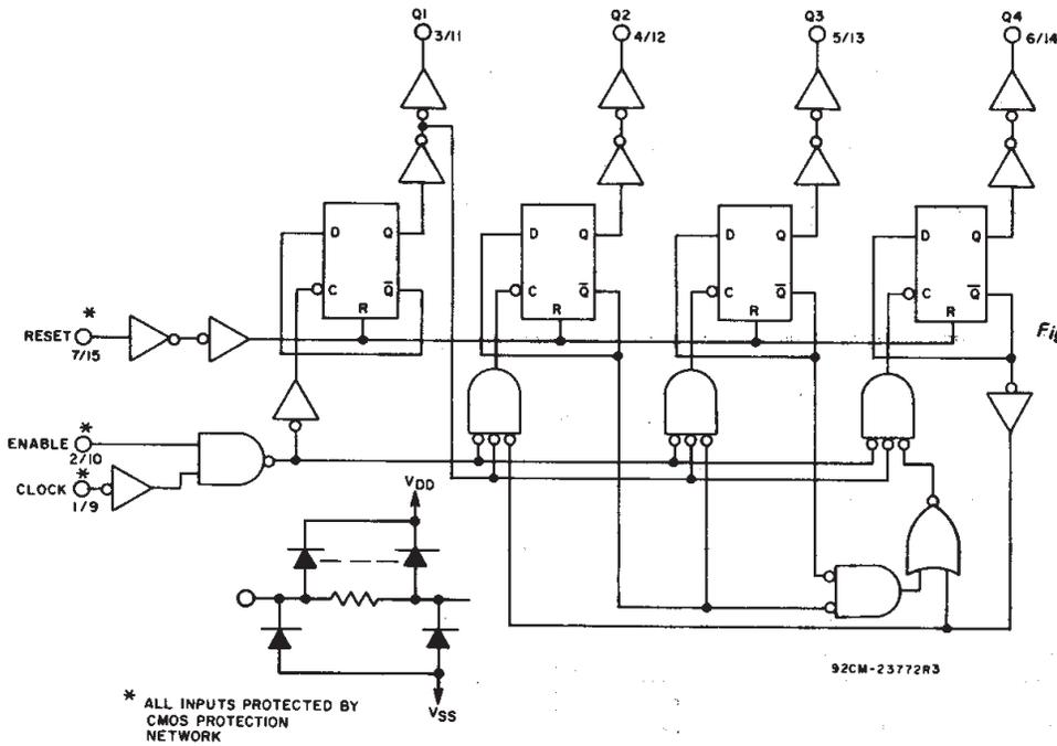
Fig. 14 — Decade counter (CD4518B) logic diagram for one of two identical counters.
