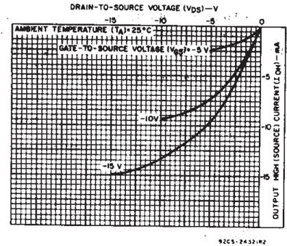
Fig. 4 — Minimum output high (source) current characteristics.
