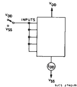
Fig. 12 - Quiescent device current test circuit.
