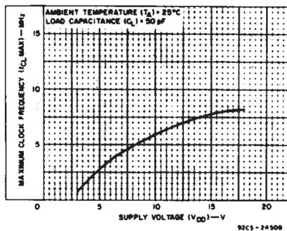
Fig. 8 — Typical maximum-clock-frequency vs. supply voltage.
