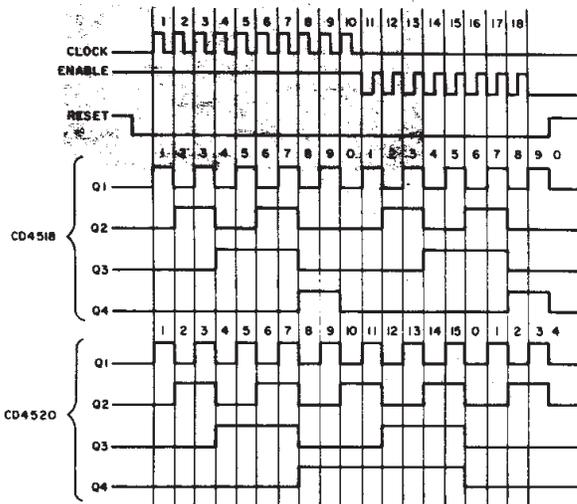
Fig. 16 — Timing diagrams for CD4518B and CD4520B.
