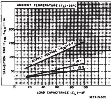
Fig. 7 — Typical transition time vs. load capacitance.
