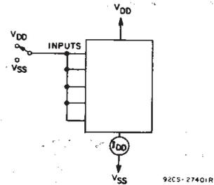
Fig. 12 - Quiescent device current test circuit.
