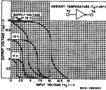
Fig. 9 - Minimum and maximum transfer characteristics - complement output.
