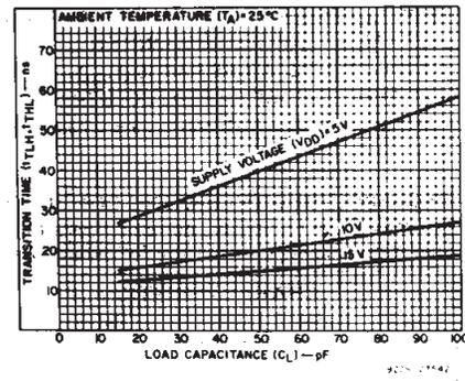
Fig. 7 - Typical transition time vs. load capacitance.
