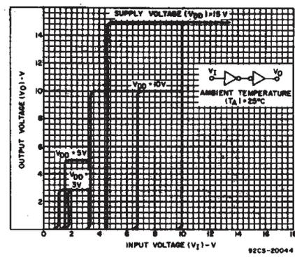
Fig. 8 - Minimum and maximum transfer characteristics - true output.
