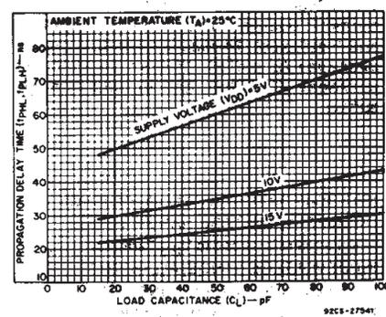
Fig. 6 - Typical propagation delay time vs. load capacitance.
