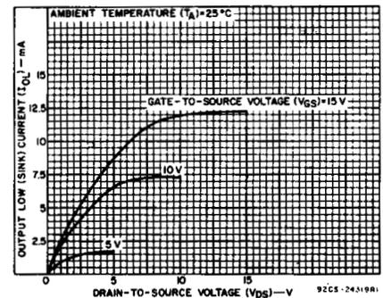
Fig. 2—Minimum n-channel output low (sink) current characteristics.
