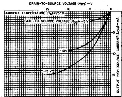
Fig. 4—Minimum p-channel output high (source) current characteristics.
