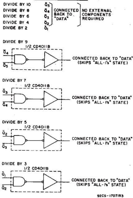
Fig. 16 — External connections for divide by 10, 9, 8, 7, 5, 4, 3, 2 operation.
