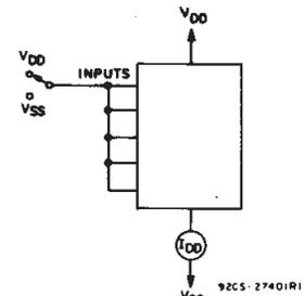
Fig. 11 — Quiescent device current test circuit.
