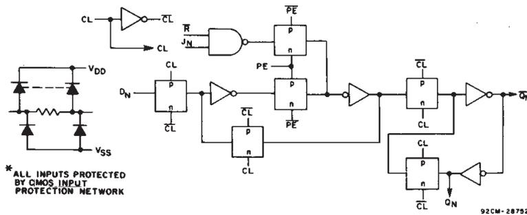
Fig. 2 - Detail of a typical stage.
