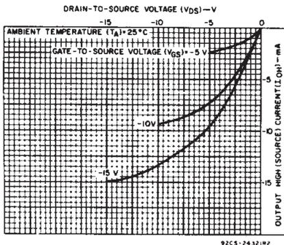
Fig. 6 - Minimum output high (source) current characteristics.
