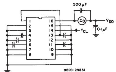
Fig. 14 — Dynamic power dissipation test circuit.
