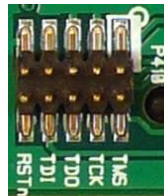
Figure 19 – 10-pin ARM Cortex Debug header (P410)
