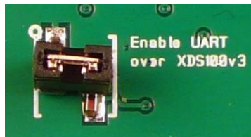
Figure 7 – Jumper mounted on J5 to enable the UART back channel
