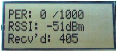
The receiver will also display the number of received packets and a moving average RSSI value based on the last 32 packets.
