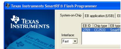
The Flash Programmer application, available on the kit web page [2], can be used to program Intel HEX files, read the contents of flash and several other operations.
