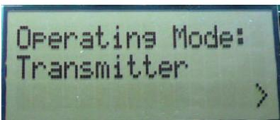
Set the other board to operate as transmitter. Use the joystick to select mode. Confirm the selection by pressing Button 1.
