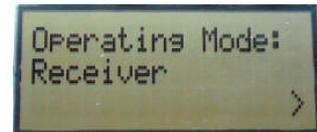
Set one of the boards to operate as receiver. Use the joystick to select mode. Confirm by pressing Button 1.
