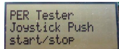
The transmitter is now configured for the PER test. The PER test is started and stopped by moving the joystick (in any direction). The transmitter will display the number of packets sent during the PER test.
