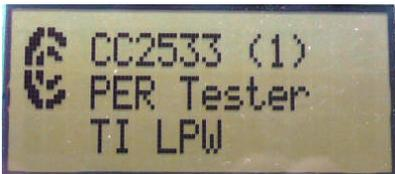
When power is applied to the SmartRF05EB, the preprogrammed PER test on the CC2533 will start running.
