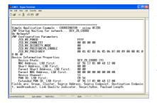
Push the button on the target board to display the status window of the network after the terminal has connected. Information about the ZNP and device is displayed. The coordinator is now ready to connect to other devices on the network. For more information about the message format, please see the Simple Application wiki page:
