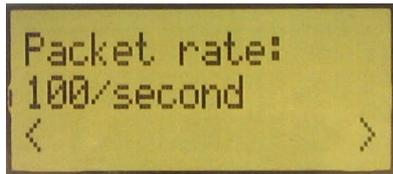
Select packet rate (number of packets transmitted per second) on the transmitter. Confirm the selection with Button S1.
