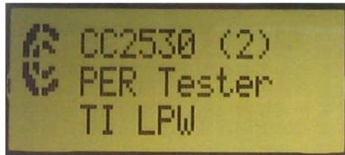
When power is applied to the SmartRF05EB, the preprogrammed PER test on the CC2530 will start running. The LCD will display the screen as shown in the picture above. The number in the parentheses is the revision of the CC2530. Press Button S1 to enter the menu.
