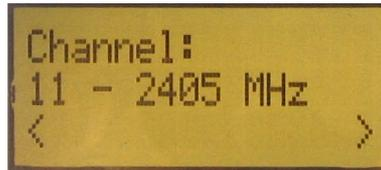
Select a channel between 11 and 26 (2405-2480 MHz). The channel is selected by navigating the joystick to the right or left. Confirm the selection by pressing Button S1.
