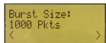
Select burst size (number of packets to send) by using the joystick, either 1000, 10K, 100K or 1M packets. Confirm the selection with Button S1.
