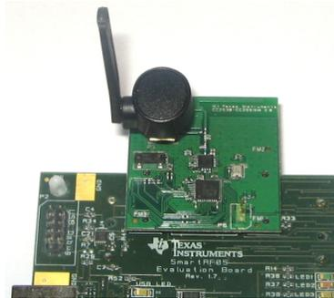
The CC2530-CC2591EM can be plugged into the SmartRF05EB. Please refer to the SmartRF05EB User Guide for more information about SmartRF05EB (<http://www.ti.com/lit/pdf/swru210>)
