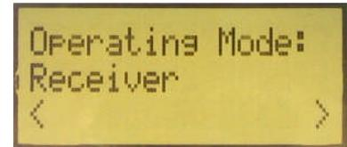
Select receiver on one of the SmartRF05EB's and transmitter on the other. Use the joystick to select mode. Confirm the selection by pressing Button S1.
