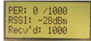
The PER test receiver will display the PER value (number of lost and erroneous packets divided by the total number of packets sent, displayed as a fraction of 1000). It will also display a moving average RSSI value (received signal strength). The test can be reset by pressing Button S1.
