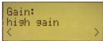
For the receiver select LNA gain on the CC2591 with the joystick. Either high gain or low gain mode are possible settings. Normally, high gain mode should be selected. Confirm the selection with Button S1. The receiver is now ready to receive packets.
