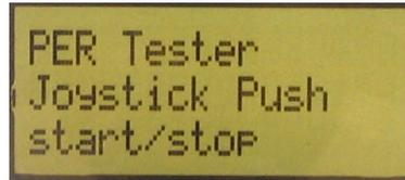
The transmitter is now configured for the PER test. The PER test is started by pushing the joystick (as a button). The transmitter will display the number of packets sent during the PER test. The PER test is stopped by pushing the joystick again.
