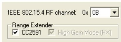
Studio will then make sure that I/O on the CC2530 is set up for proper control of the CC2591.
