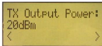
On the transmitter node, select the TX output power (signal strength). Use the joystick to select between 0 dBm, 13 dBm, 16 dBm, 18 dBm or 20 dBm. Confirm the selection with Button S1.
