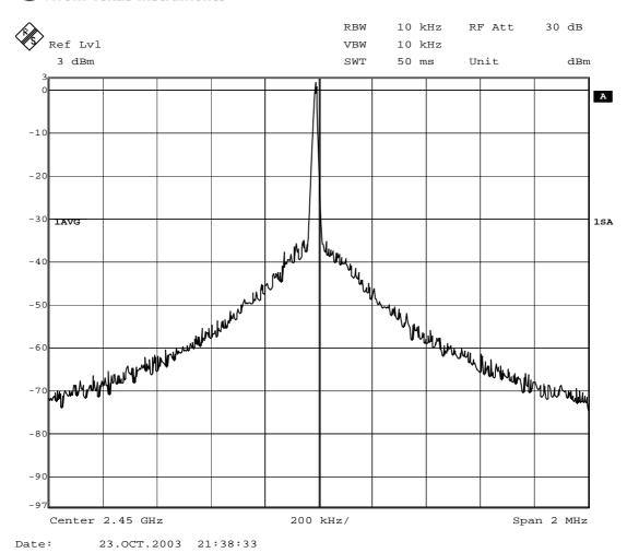
Figure 31. Single carrier output
