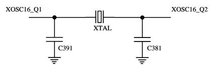
Figure 30. Crystal oscillator circuit
