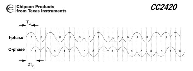
Figure 7. I / Q Phases when transmitting a zero-symbol chip sequence,  $T_c = 0.5 \ \mu s$
