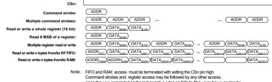
since they are completed on the last negative edge on SCLK. They may however also be terminated with setting CSn high, if desirable, e.g. for reading only 8 bits from a configuration register.
