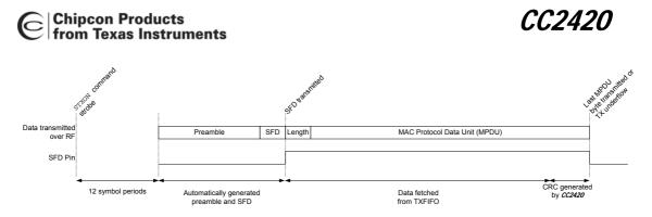
Figure 15. Pin activity example during transmit
