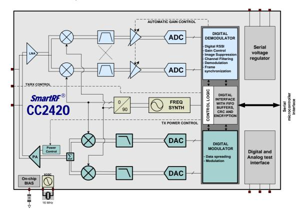
Figure 2. CC2420 simplified block diagram
