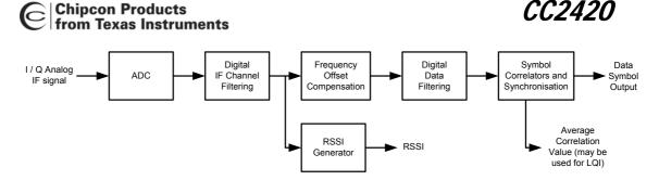
Figure 16. Demodulator Simplified Block Diagram
