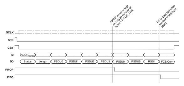
Figure 14. Example of pin activity when reading RXFIFO.
