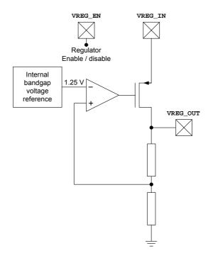
Figure 28. Voltage regulator, simplified schematic
