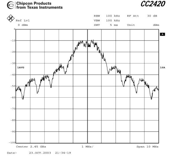
Figure 32. Modulated spectrum plot
