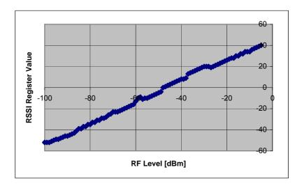
Figure 27. Typical RSSI value vs. input power
