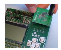
Insert a CC1125EM board into the TrxEB as shown above. Connect the antenna to the SMA connector on the EM.
