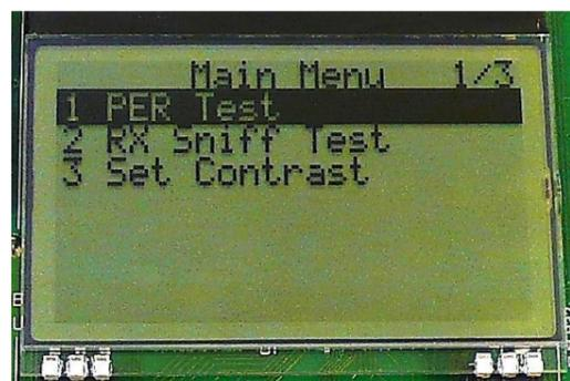
Select the PER (Packet Error Rate) test by highlighting the selection using the up/down buttons. Confirm your selection by pressing Enter (right button).
