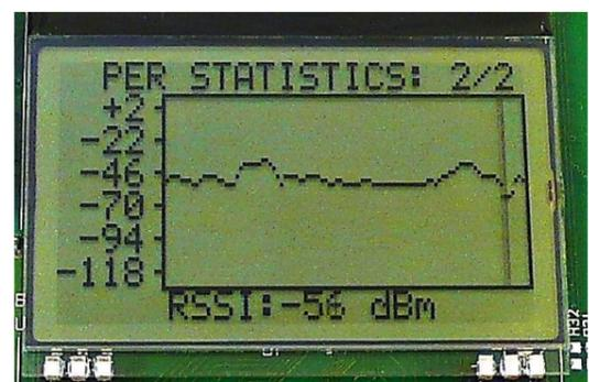
When selecting "Start PER Test", the master (receiver) will begin to count the number of received packets and provide some statistics.
