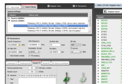
You can now configure the radio, run performance tests, export register settings and run link tests with another CC1120 or C1121 on a SmartRF TrxEB connected to the PC.
