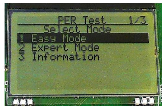
The PER test can be run in several modes. Easy Mode sets up a one-way test and uses default settings. This test is convenient for practical range testing.
