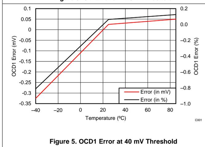
**Figure 5. OCD1 Error at 40 mV Threshold**
