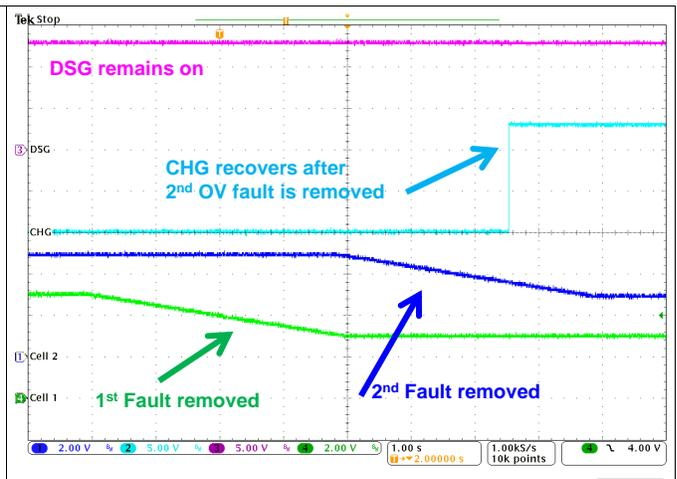
Figure 29. OV Fault Recovery
