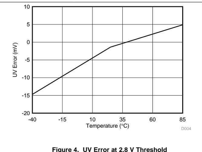
**Figure 4. UV Error at 2.8 V Threshold**
