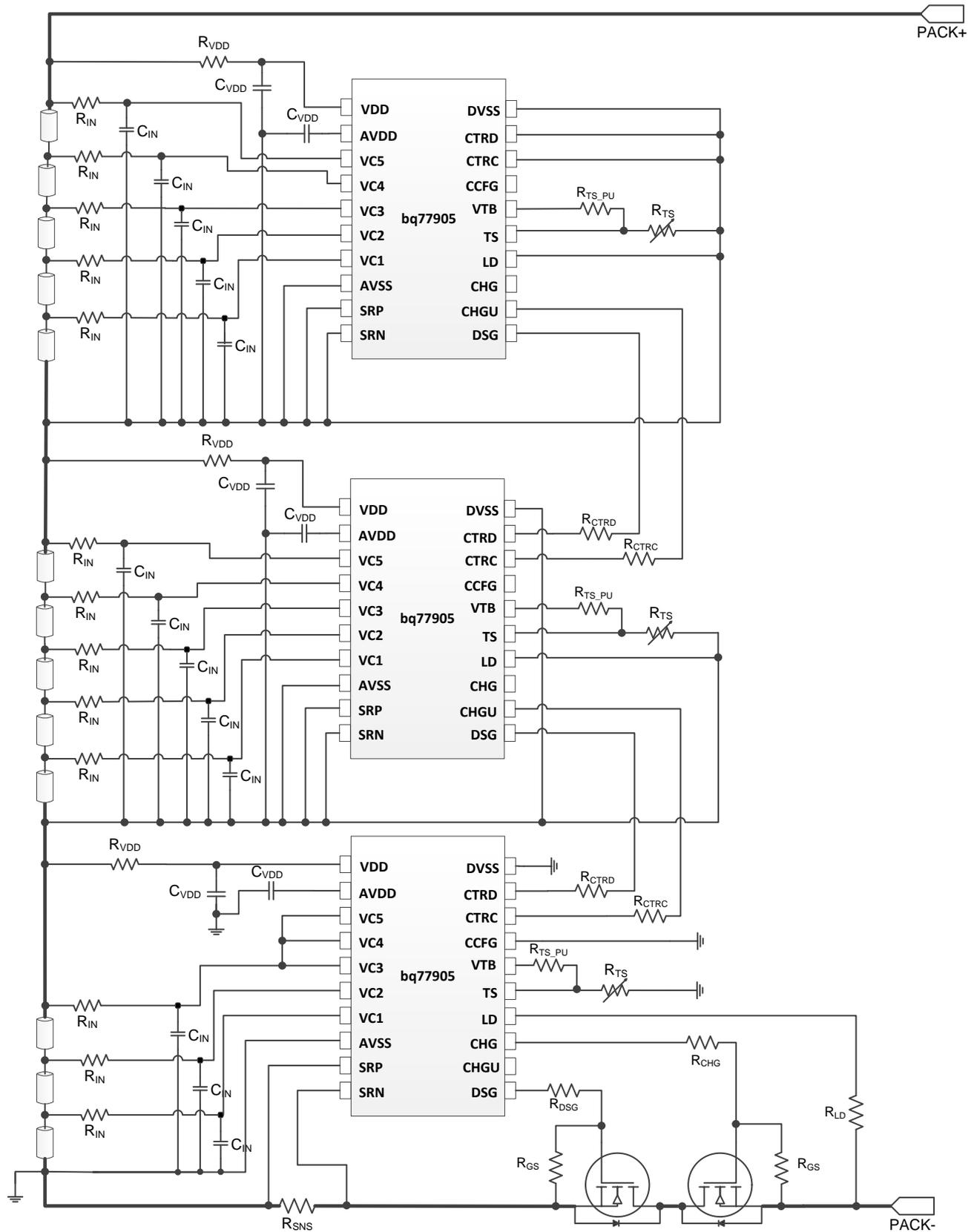
Figure 18. 13S Pack Using Three bq77905 Devices
