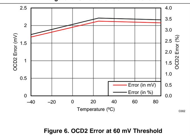
**Figure 6. OCD2 Error at 60 mV Threshold**
