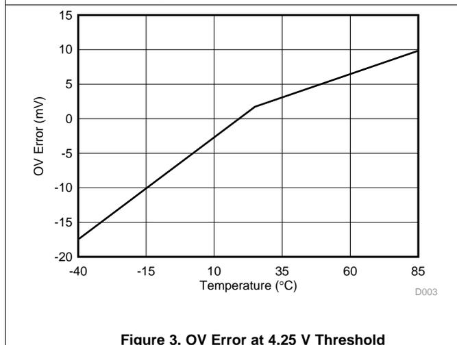
**Figure 3. OV Error at 4.25 V Threshold**
