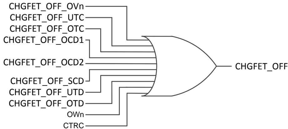
Figure 15. Faults That Can Qualify CHGFET OFF
