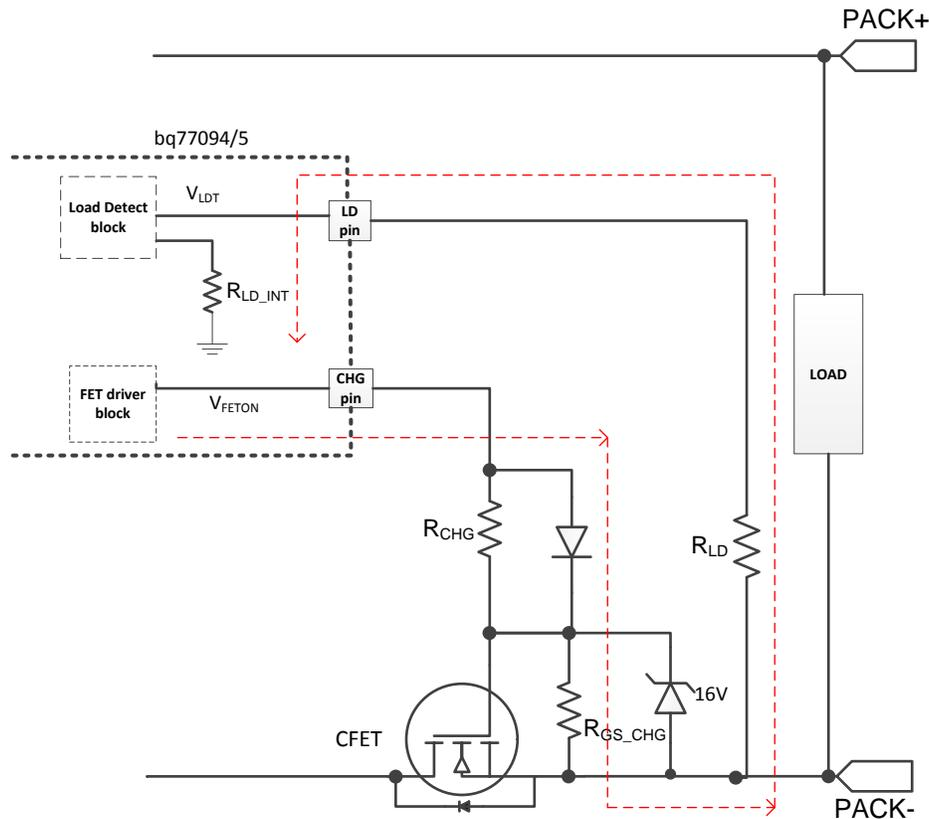
Figure 24. Load Detect Circuit During UV Fault
