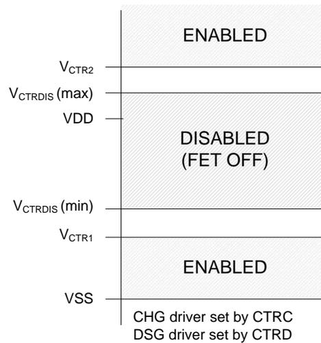
**Figure 16. External Override of CHG and DSG Drivers**
