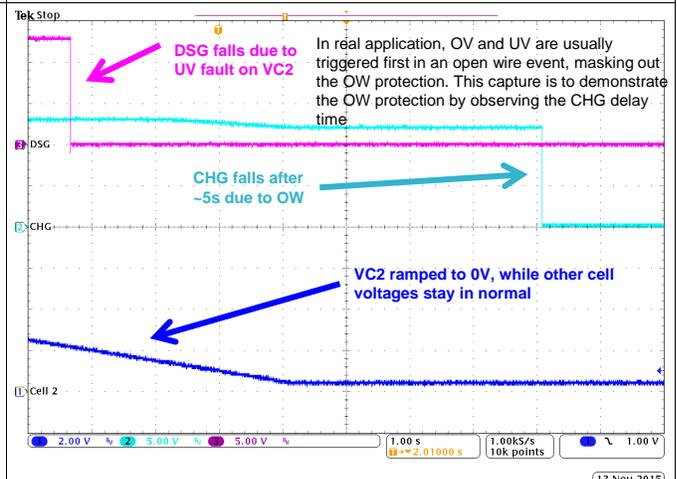
Figure 33. OW Fault Protection - Ramping Down Cell2 Voltage
