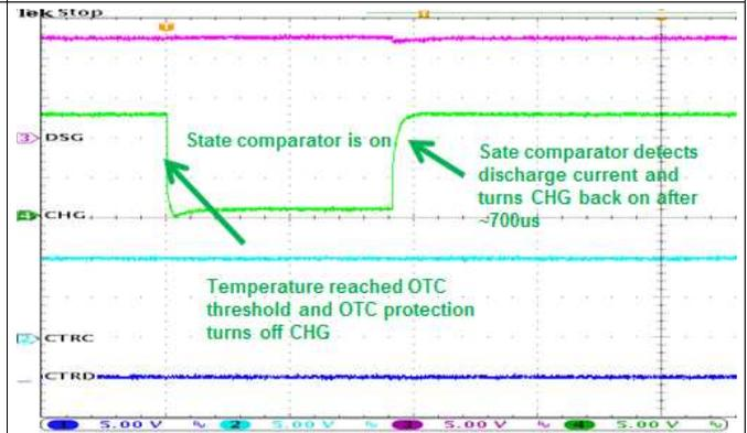
Figure 31. Detect OTC Fault While in 30A Discharge
