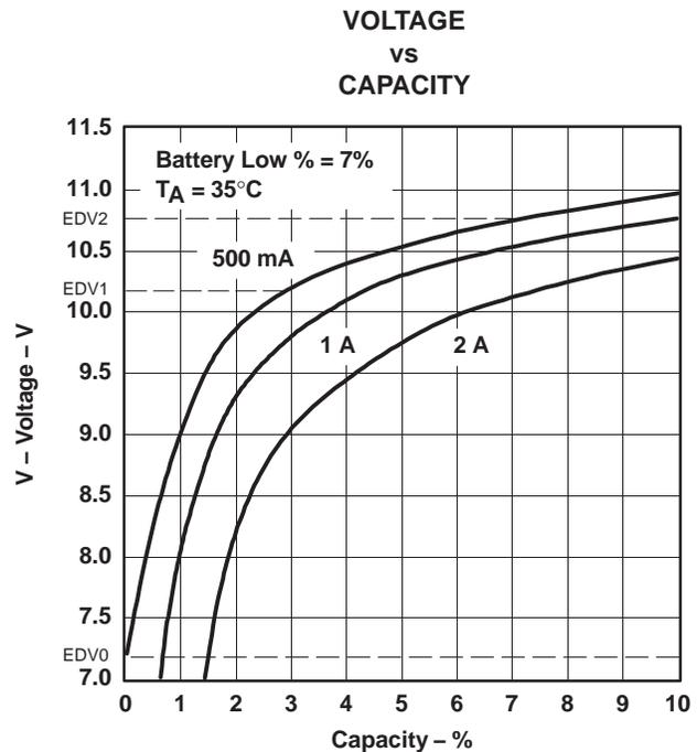
Figure 9. EDV Calculations vs Capacity for Various Loads
