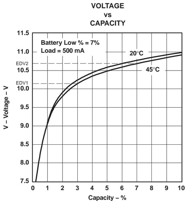
Figure 8. EDV Calculations vs Capacity for Various Temperatures
