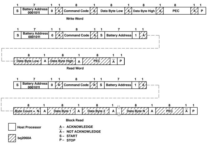
Figure 9. SMBus Communication Protocol with PEC
