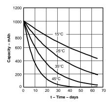
Figure 7. Self-Discharge at 2.5%/Day at 25°C
