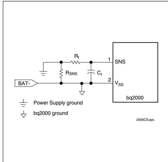
**Figure 9. Current-Sensing Circuit**
