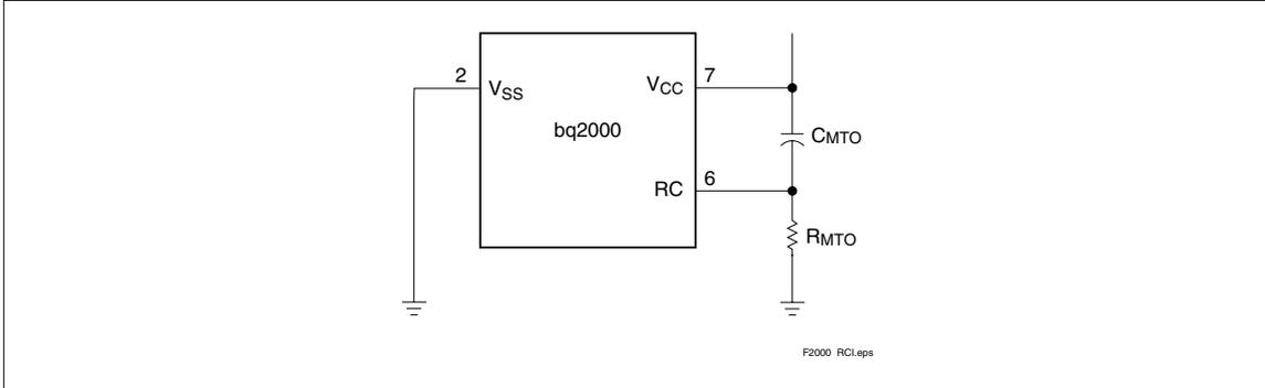
Figure 4. Typical Connection for the RC Input
