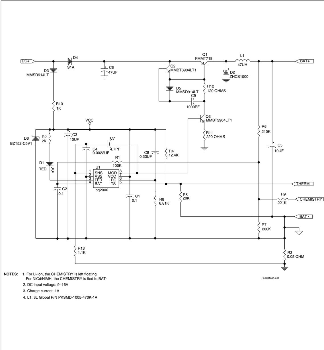
Figure 8. Single-Cell Li-Ion, Three-Cell NiCd/NiMH 1A Charger
