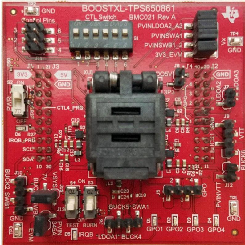
Figure 2. BOOSTXL-TPS650861 BoosterPack™ Plug-in Module
