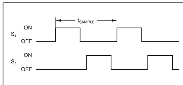
Figure 36.  $S_1$  and  $S_2$  Switch Timing for Figure 37
