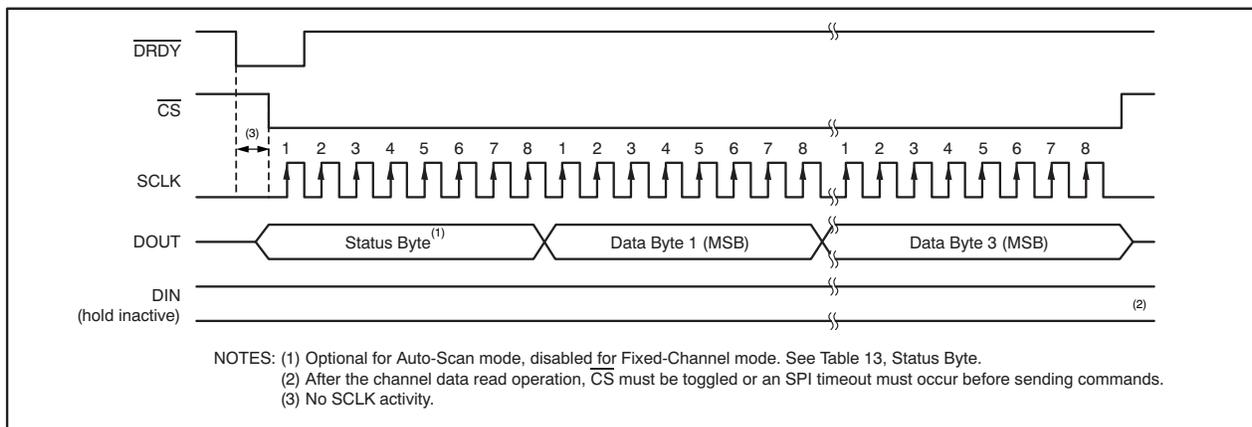
Figure 57. Channel Data Read Direct (No Command)
