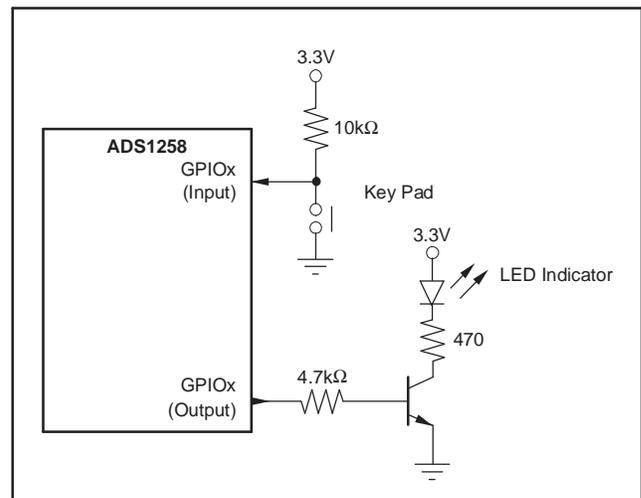
Figure 66. GPIO Connections
