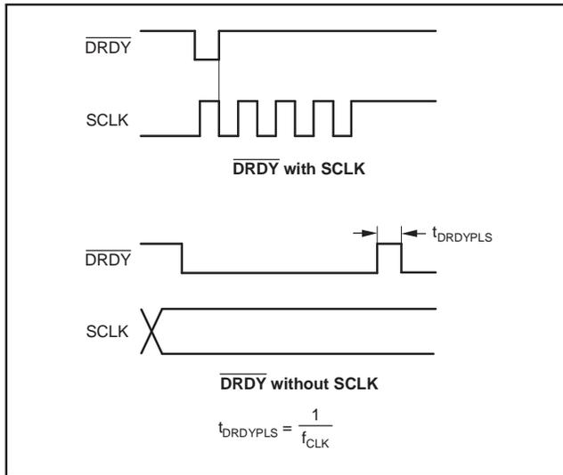
**Figure 52.  $\overline{\text{DRDY}}$  Timing**
