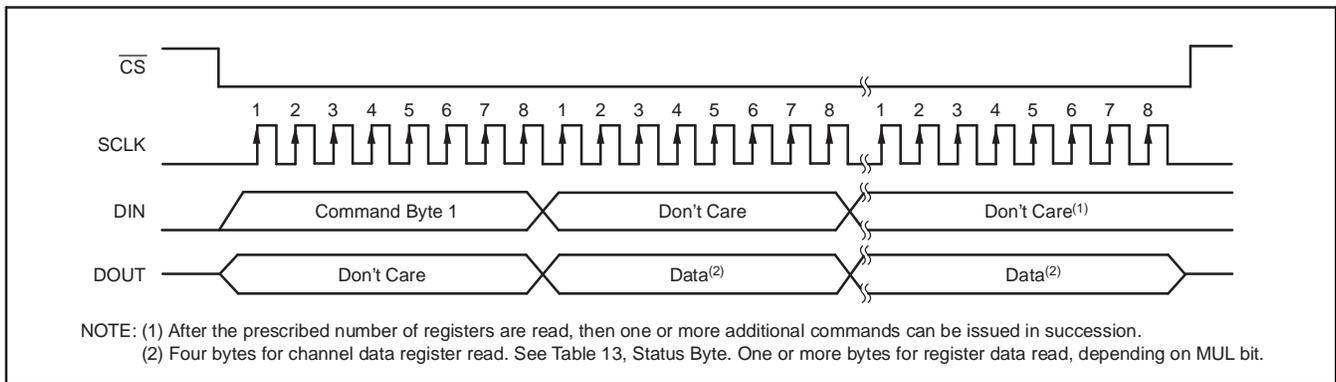
**Figure 58. Register and Channel Data (Register Format) Read**
