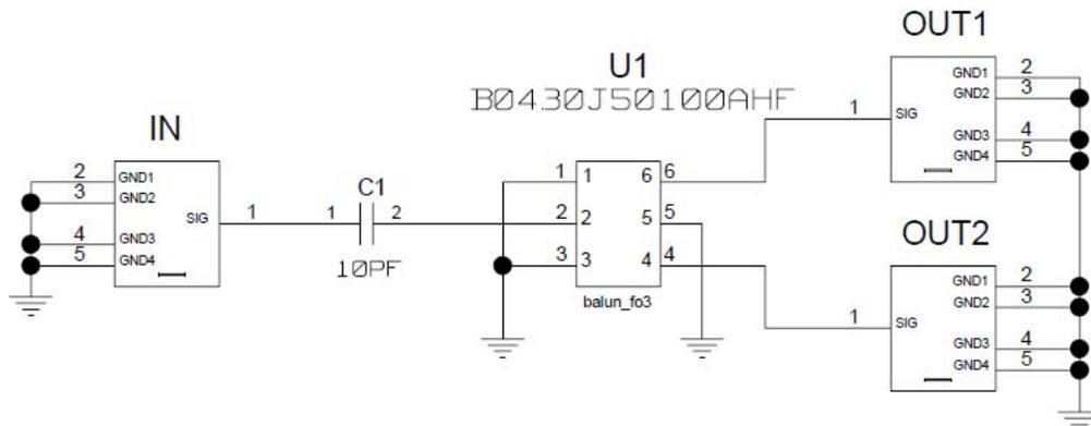
Figure 2. ADC-LD-BB Schematic
