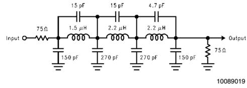
**FIGURE 8. 11 MHz Low Pass filter to eliminate harmonics at the signal input.
