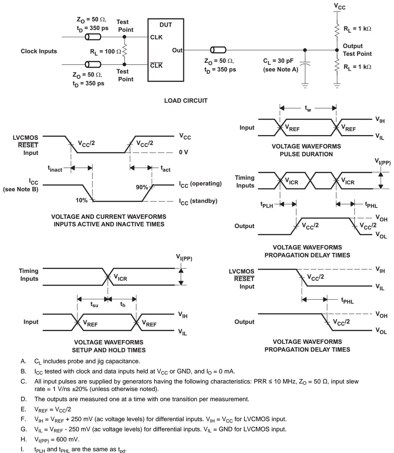
**Figure 2. Data Output Load Circuit and Voltage Waveforms**
