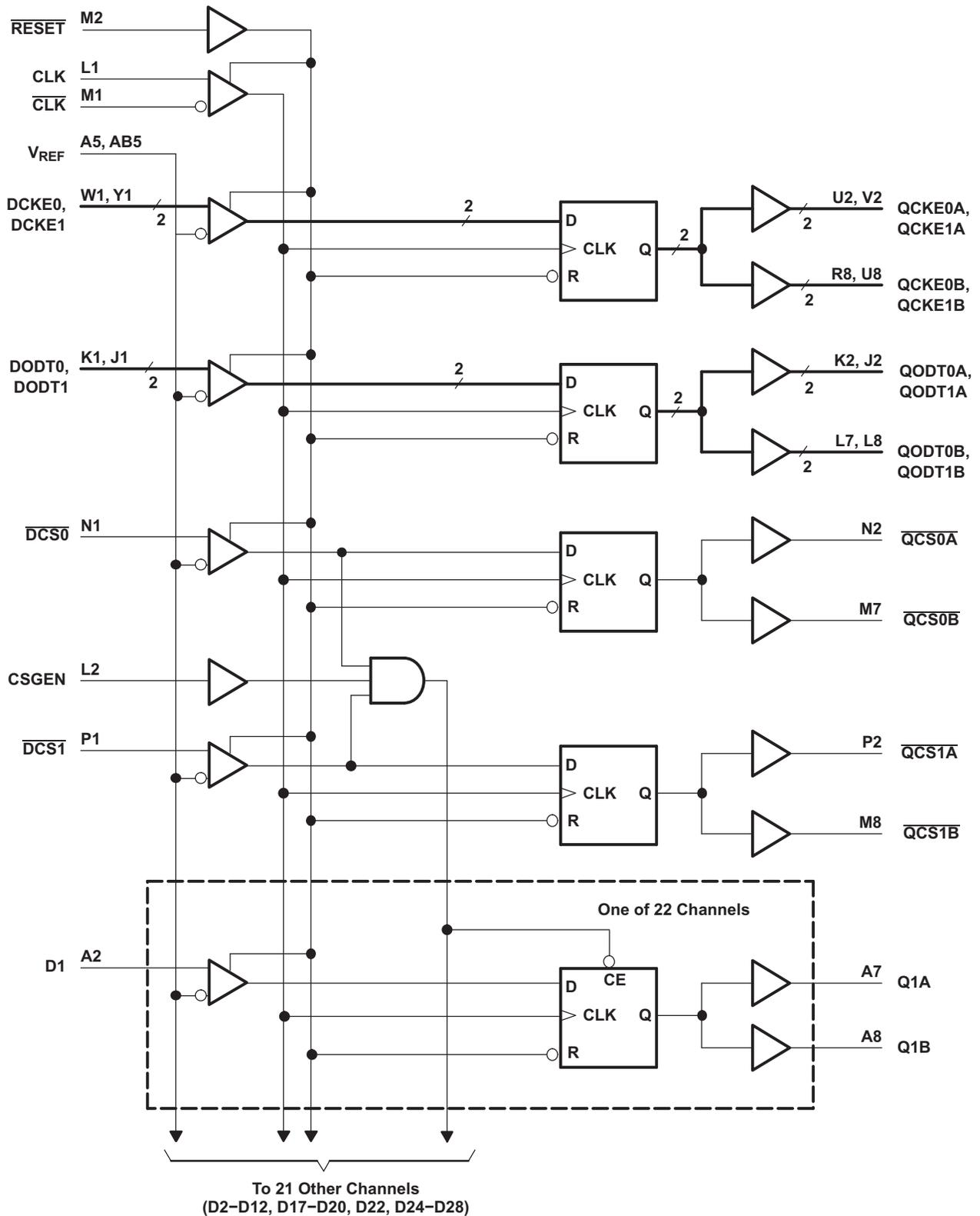
Parity Logic Diagram for Register-B Configuration (Positive Logic); C = 1
