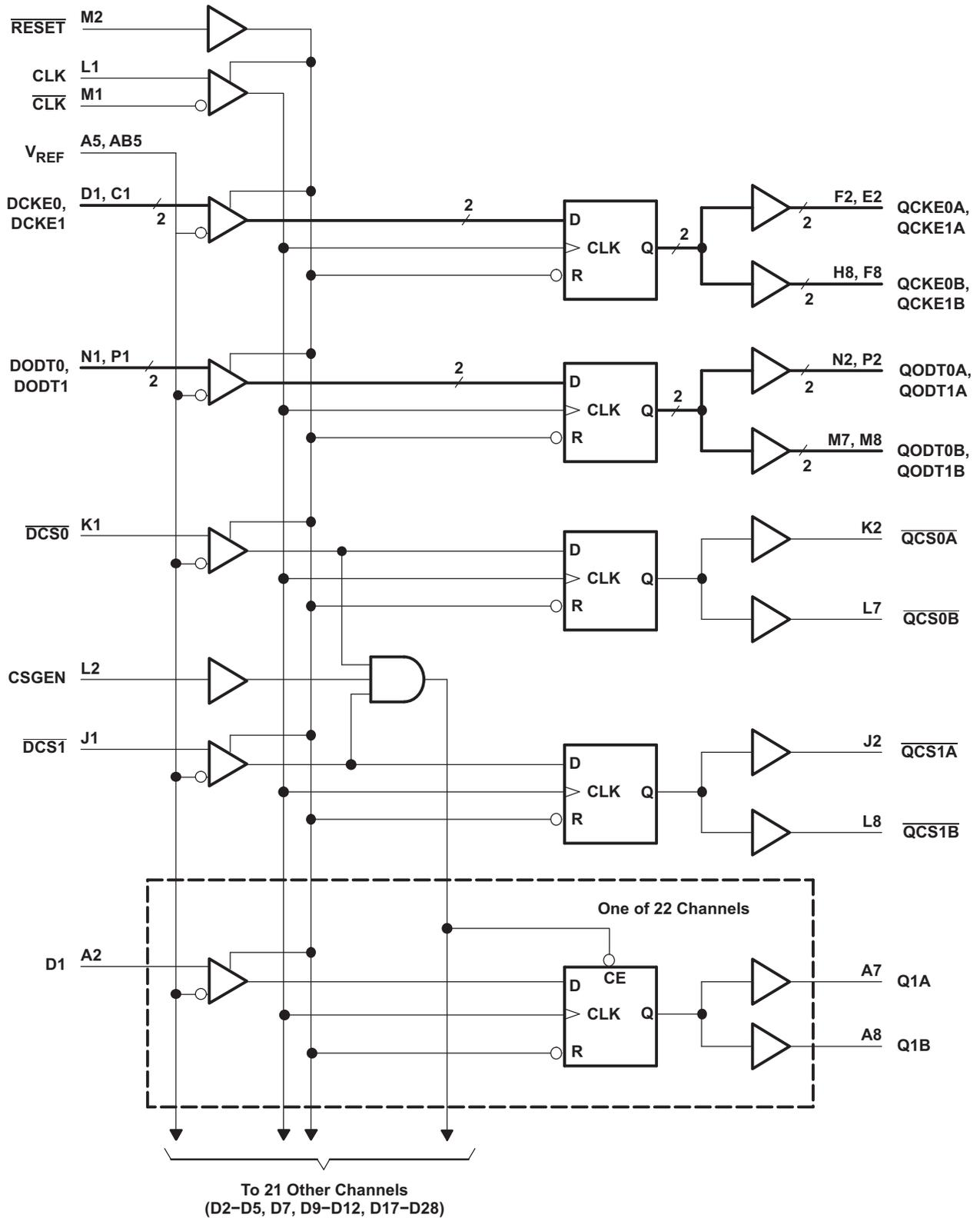
Parity Logic Diagram for Register-A Configuration (Positive Logic); C = 0
