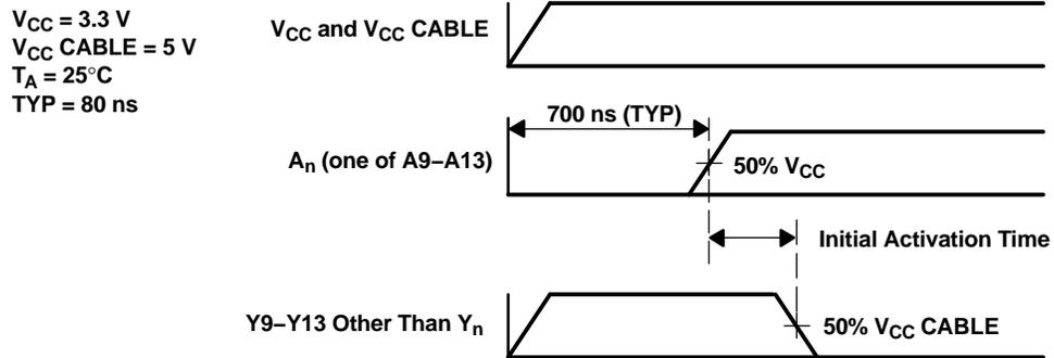
NOTE A: One of A9–A13 is switched as shown above, and the other four inputs are forced to low state.
