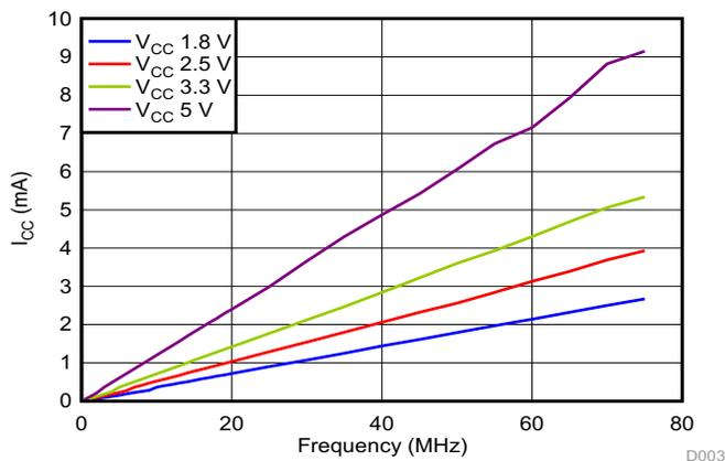
Figure 6. I<sub>CC</sub> vs Frequency
