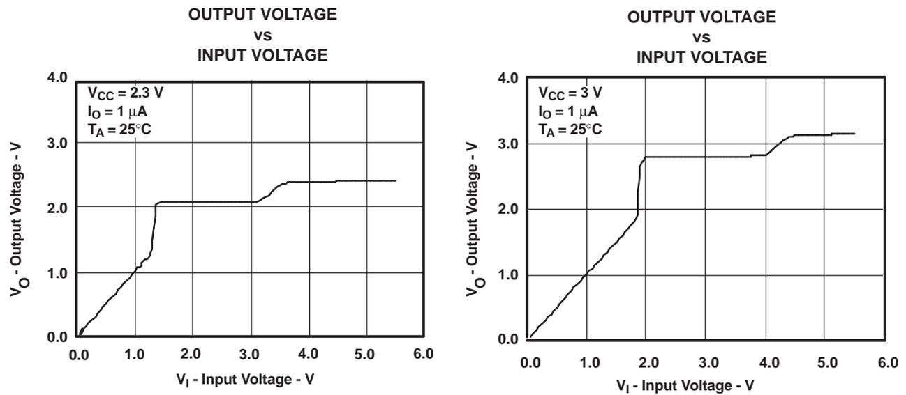
Figure 3. Data Output Voltage vs Data Input Voltage
