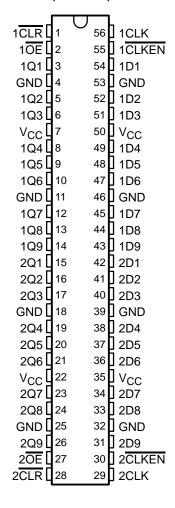
A buffered output-enable (OE) input can be used to place the outputs in either a normal logic state (high or low logic levels) or a high-impedance state. In the high-impedance state, the outputs neither load nor drive the bus lines significantly.
