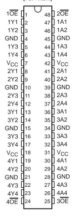
The 74ACT16244 is packaged in TI's shrink small-outline package, which provides twice the I/O pin count and functionality of standard small-outline packages in the same printed-circuit-board area.
