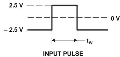
A. Figure 11 shows the maximum duration of the illustrated pulse that can be applied differently without the output changing from the low to high level.
