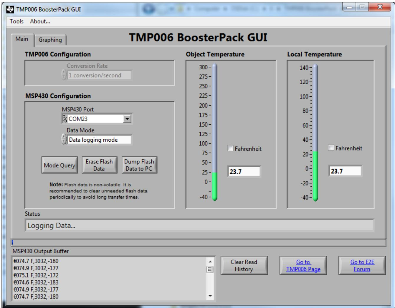
**Figure 8. BoosterPack GUI in Data Logging Mode**
