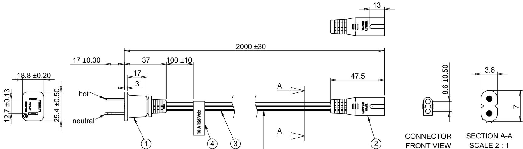
Wire marking: (UL) E339575 SPT-2 2X0.824mm2
