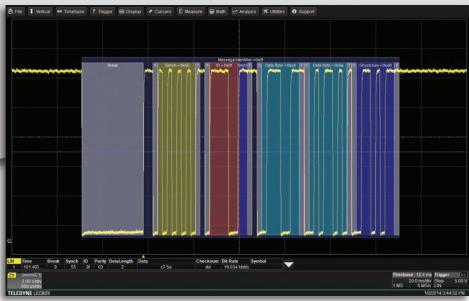
Trigger on exactly the message packets you want with powerful conditional DATA triggering. Apply a color-coded, easy-to-understand, decode over your LIN messages. Search for and find specific message packets in long acquisitions.
