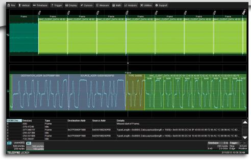
Ethernet decoding provides protocol awareness to the oscilloscope for fast debugging.
