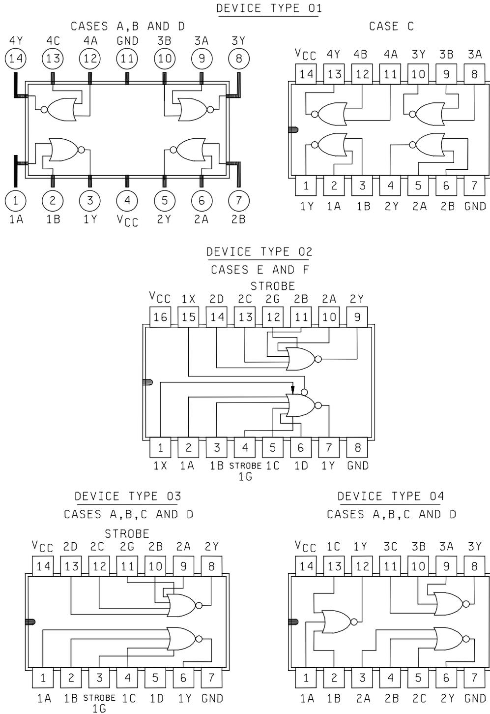
Figure 1. Logic diagram and terminal connections (top view).
