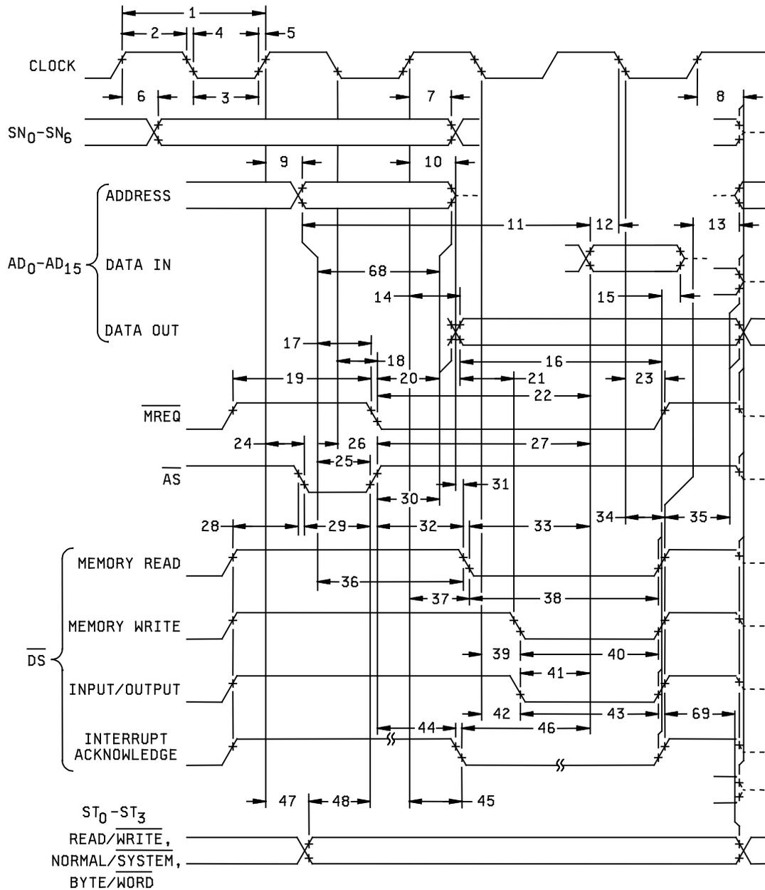
FIGURE 4. Timing waveforms.
