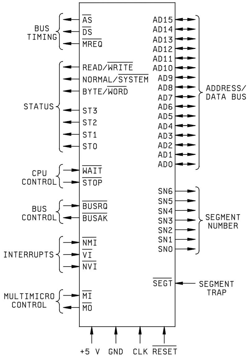
FIGURE 3. Logic functions.
