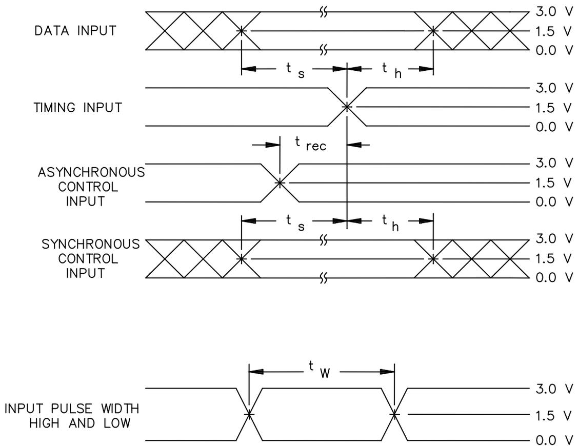
FIGURE 5. Switching waveforms and test circuit.
