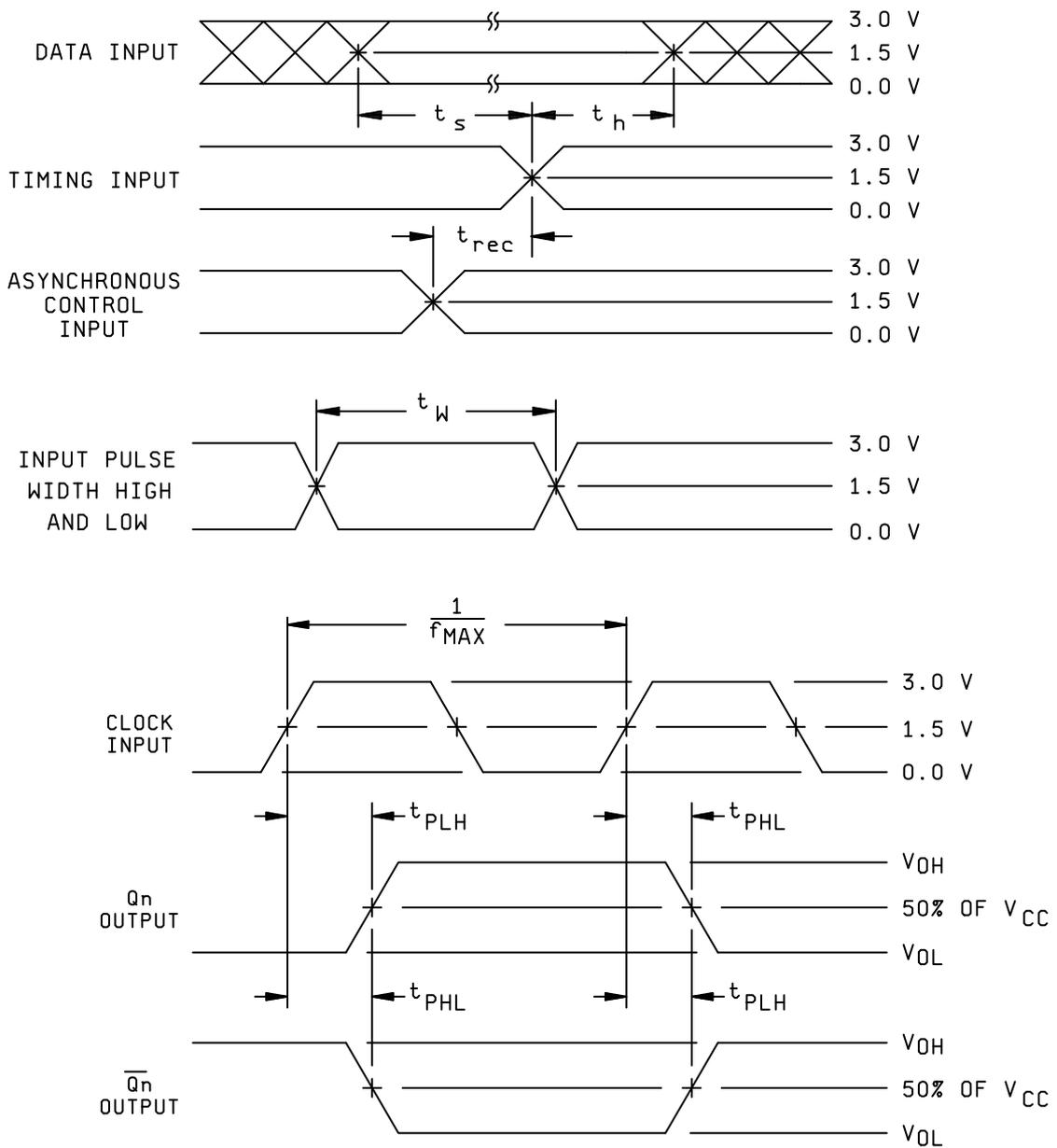
FIGURE 5. Switching waveforms and test circuit.
