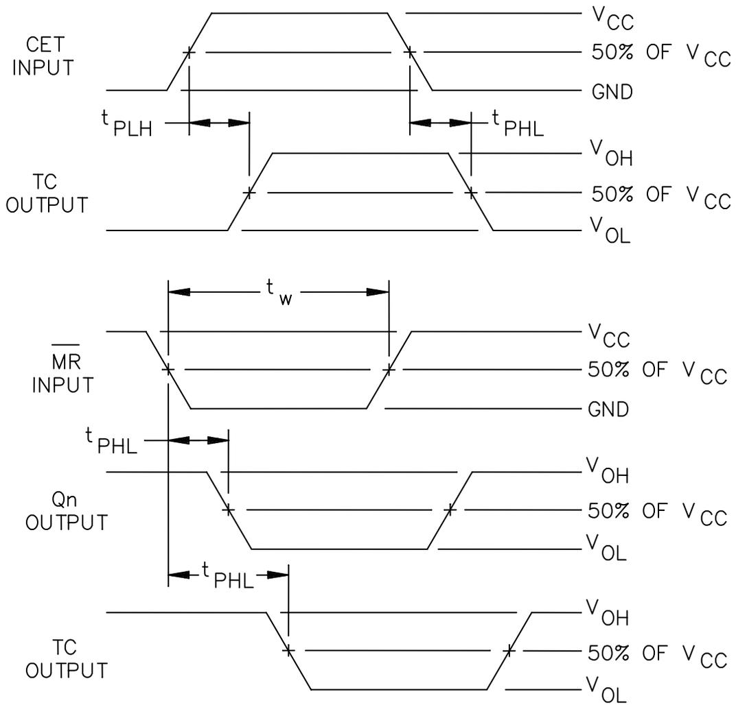
FIGURE 5. Switching waveforms and test circuit - Continued.
