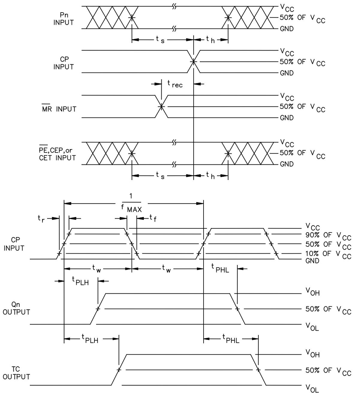
FIGURE 5. Switching waveforms and test circuit.
