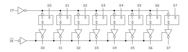
FIGURE 3. Logic diagram.
