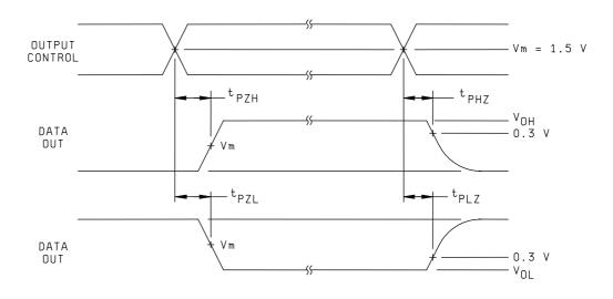
FIGURE 4. Switching waveforms and test circuit.
