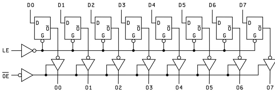
FIGURE 3. Logic diagram.
