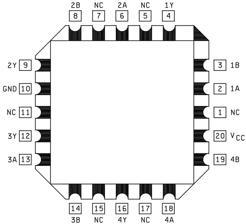
FIGURE 1. Terminal connections and logic diagram.
