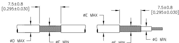
“G” is the minimum diameter on which the sleeve will seal.
