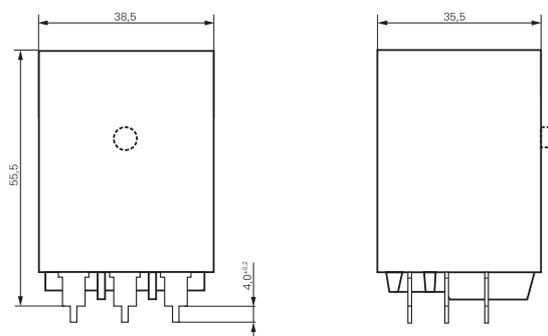
Cover with mounting brackets, 6.3mm quick connect (4.8mm available)
