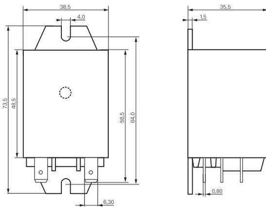
Cover with DIN-snap-on attachment (6.3mm quick connect only)
