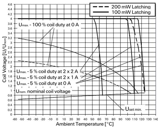
All figures are given for coil without pre-energization, at ambient temperature +23°C.
