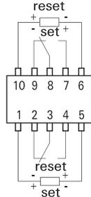
Contacts are shown in reset condition. Both coils can be used as either set or reset coils. Contact position might change during transportation and must be reset before use.
