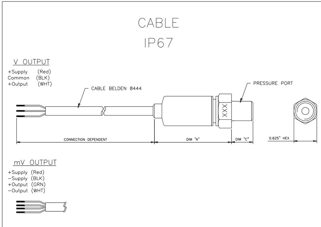
Note: Mating connector is available with 3FT of cable P/N(2001140-03)
