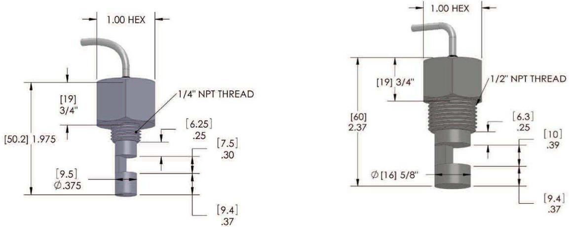
Figure 1: Left - LL-01 series element with 1/4" NPT sensor mounting
