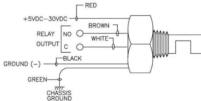
Figure 2: Typical wiring diagram for LL-01 series elements
