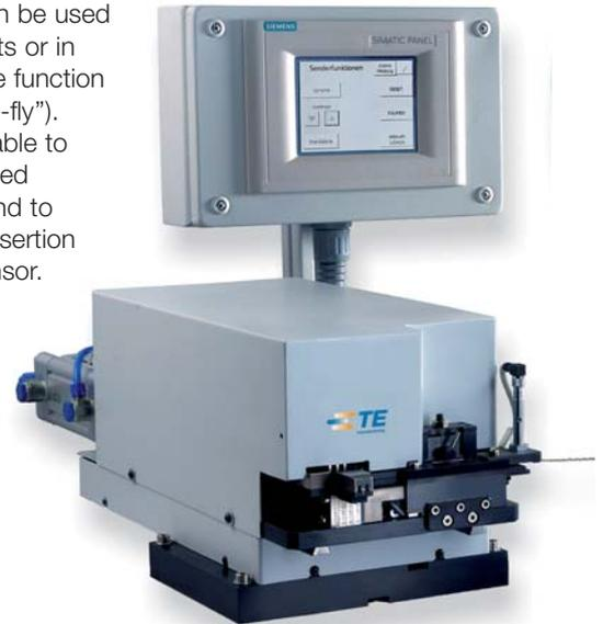
**Pneumatic Insertion Tool for MAG-MATE Terminals**
