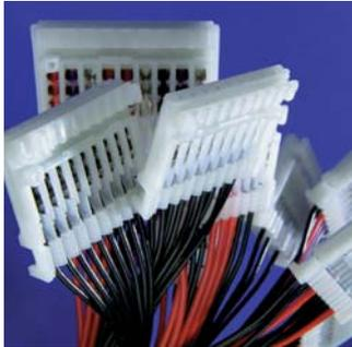
The IDC workstation produces electrical connections for harness assemblies specifically intended for the use within dashboard applications in the automotive industry. The proven insulation displacement technology ensures a high level of reliability. The software allows the production of different harness configurations featuring up to 11 connectors. The workstation is compatible with IDC connectors with a 2.54 mm and a 3.5 mm pitch. It is intended for medium to large volume production.
