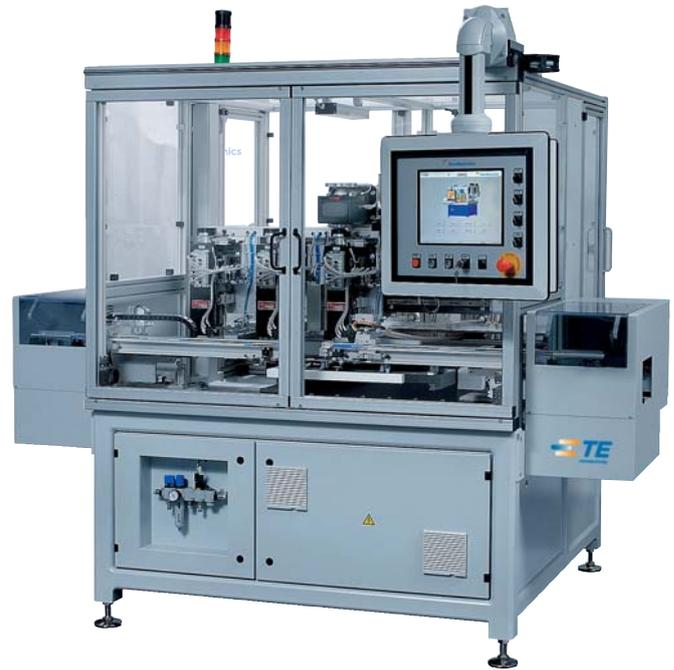
designed for easy use and provides the insertion force and a variety of production data to be collected at an open interface. With a maximum insertion rate of 4.5 cycles per
