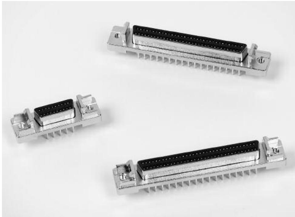
Shielded AMPLIMITE .050 Series headers with ACTION PIN contacts offer a high-density D type interface, and a solderless board-mount interconnection. These vertical mount headers are available in 20, 26, 50, 68 and 100 contact sizes. Choice of configurations includes; headers with rails and latch blocks, with latch blocks only, and without rails and latch blocks.
