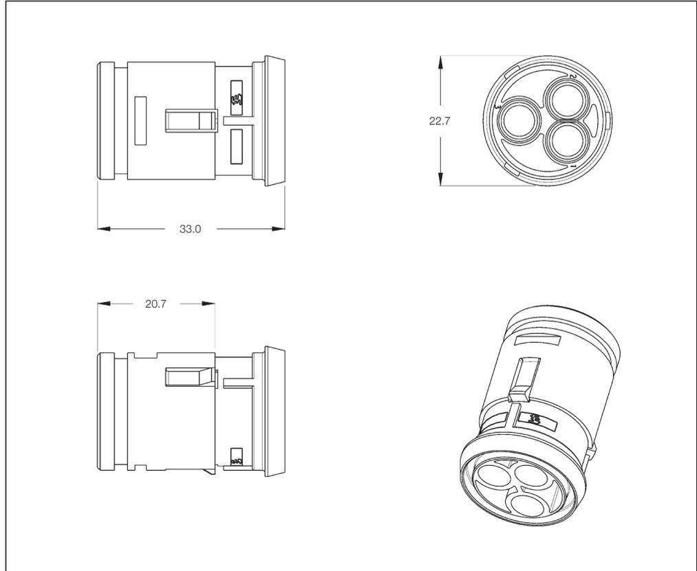
3 Position Housings for 4.0 mm Socket Contact M27 Version
