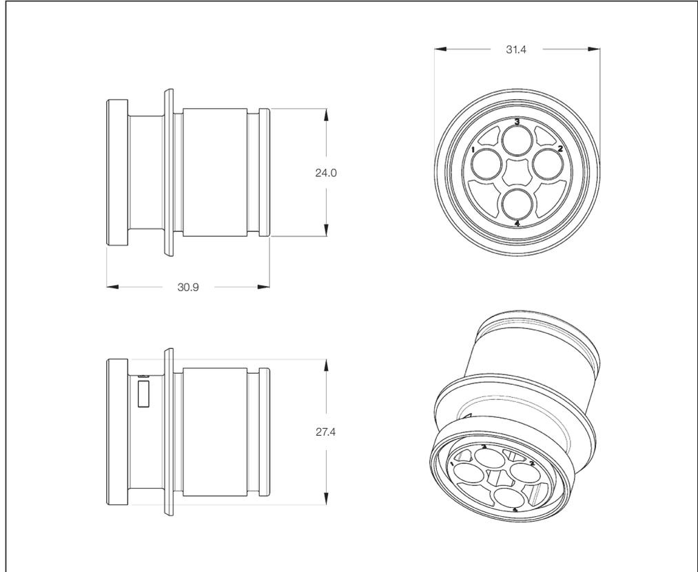
4 Position Housings for 4.0 mm Socket Contact M27 Version
