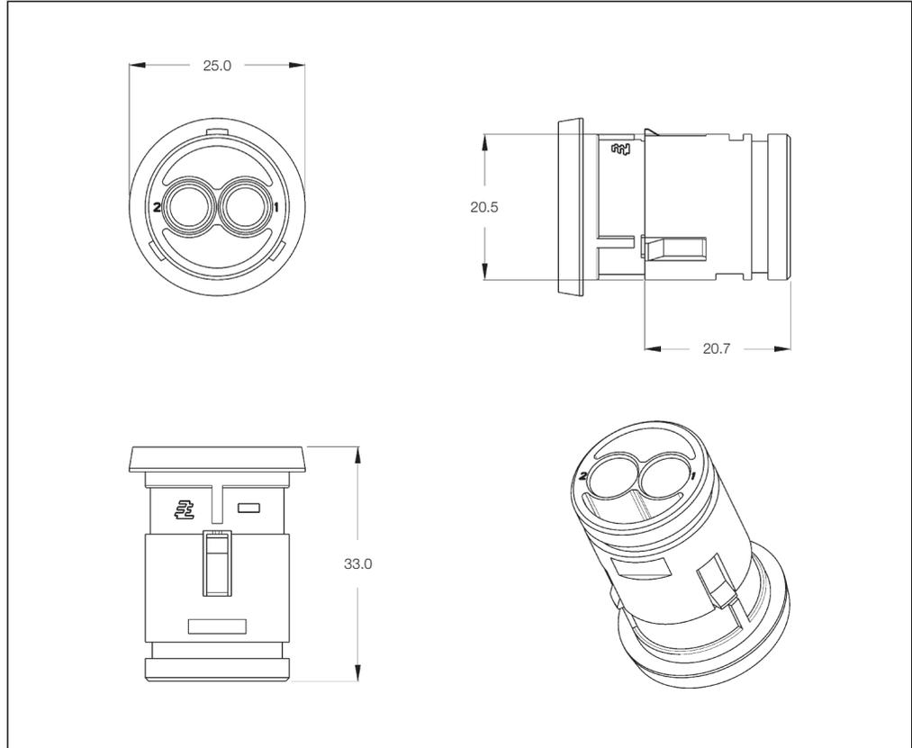
2 Position Housings for 4.0 mm Socket Contact M27 Version
