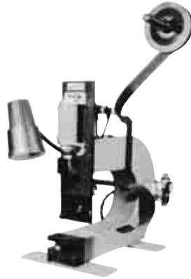
These insertion machines install contacts into printed circuit boards at rates to 2000 per hour. A spotlight highlights the insertion area and a lower tooling assures precise board location. The machines are actuated by a foot pedal and are bench mounted.
