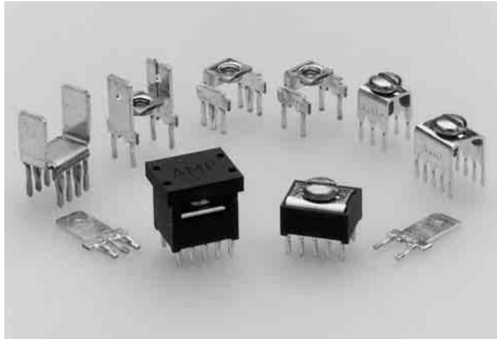
Tyco Electronics Power Taps are designed for the growing need for power to printed circuit board applications required in today's electronic industry. The taps provide a high current, separable connection to a pc board. Pin configuration is of the standard DIP outline with .300 x .100 [7.62 x 2.54] or .250 x .125 [6.35 x 3.18] for the Standard versions, plus .400 x .200 [10.16 x 5.08], .300 x .100 [7.62 x 2.54] and in-line spacing for the High Current versions.
