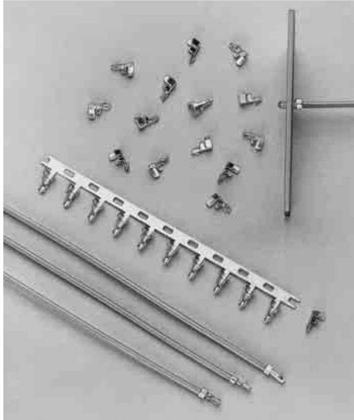
The miniature AMP-IN Terminal is designed not as an electrical terminal but as a mechanical holding device to enhance soldering of hookup wires to printed circuit boards. The combination of terminal and application tooling eliminates costly manual preparation of wires prior to soldering, and positions the wire to achieve reliable solder joints. Movement of the wire during soldering is restricted, providing for proper solder flow.
