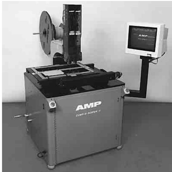
Microprocessor-controlled X-Y positioning table inserts a variety of products into pc boards, including .025<sup>2</sup> stamped or bandoliered posts, mini-spring sockets, and FASTON tabs. Insertion heads for various products are interchangeable, and can be used with bench machines. Controlled, programmed and operated using an interactive touch-screen. Options include double-action clinch tooling, powered dereeler, splice run-out detector, take-up winder for paper tape, and scrap chopper.
