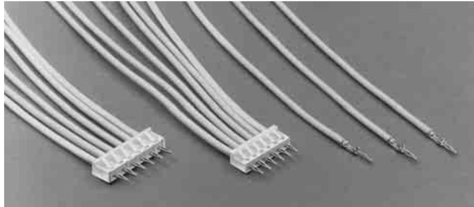
Low Profile Miniature AMP-IN Connectors provide an easy means of gang inserting leads into printed circuit boards. The design of the crimp snap-in contact aids in locating the pc board hole and inserting the contact into that hole.
