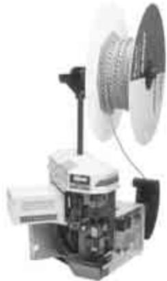
Semiautomatic bench machines for crimping reeled terminals and contacts, featuring a quiet and reliable direct motor drive, microprocessor controls for ease of setup and operation, and guarding and lighting designed for operator convenience. All models are equipped with either manual or automatic precision adjustment of crimp height. Machine-mounted sensors are available for crimp quality monitoring using conventional miniature-style applicators.
