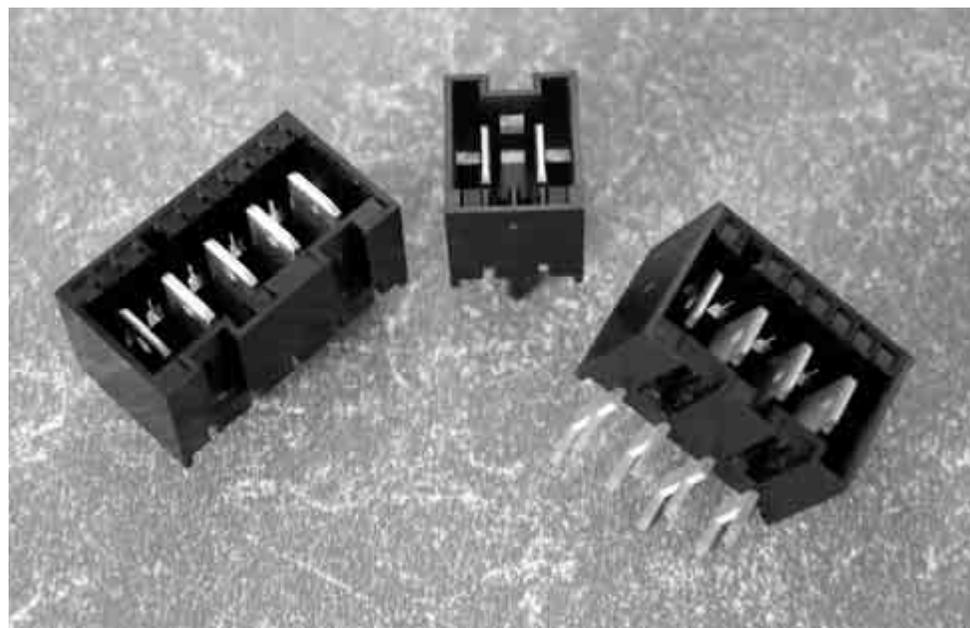
The FASTON RAST 5 Tab Header Assembly system is designed to provide a RAST 5 interface to a Printed Circuit Board. The RAST 5 Standard defines and standardizes the connector mating interface. 250 Series Tabs are placed on 5mm center lines with a plastic shroud that has keying, polarization, and locking features that help prevent mismatching of the corresponding RAST 5 female receptacle housing. The header assembly is
