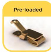
Pre-loaded spring fingers are recommended when a stable electrical contact with minimal deflection is needed. The force change is minimized over the working range of the spring finger. Pre-loaded spring fingers are available in three scalable families.
