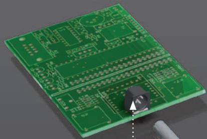
• SMD mount for soldering direct on drive
