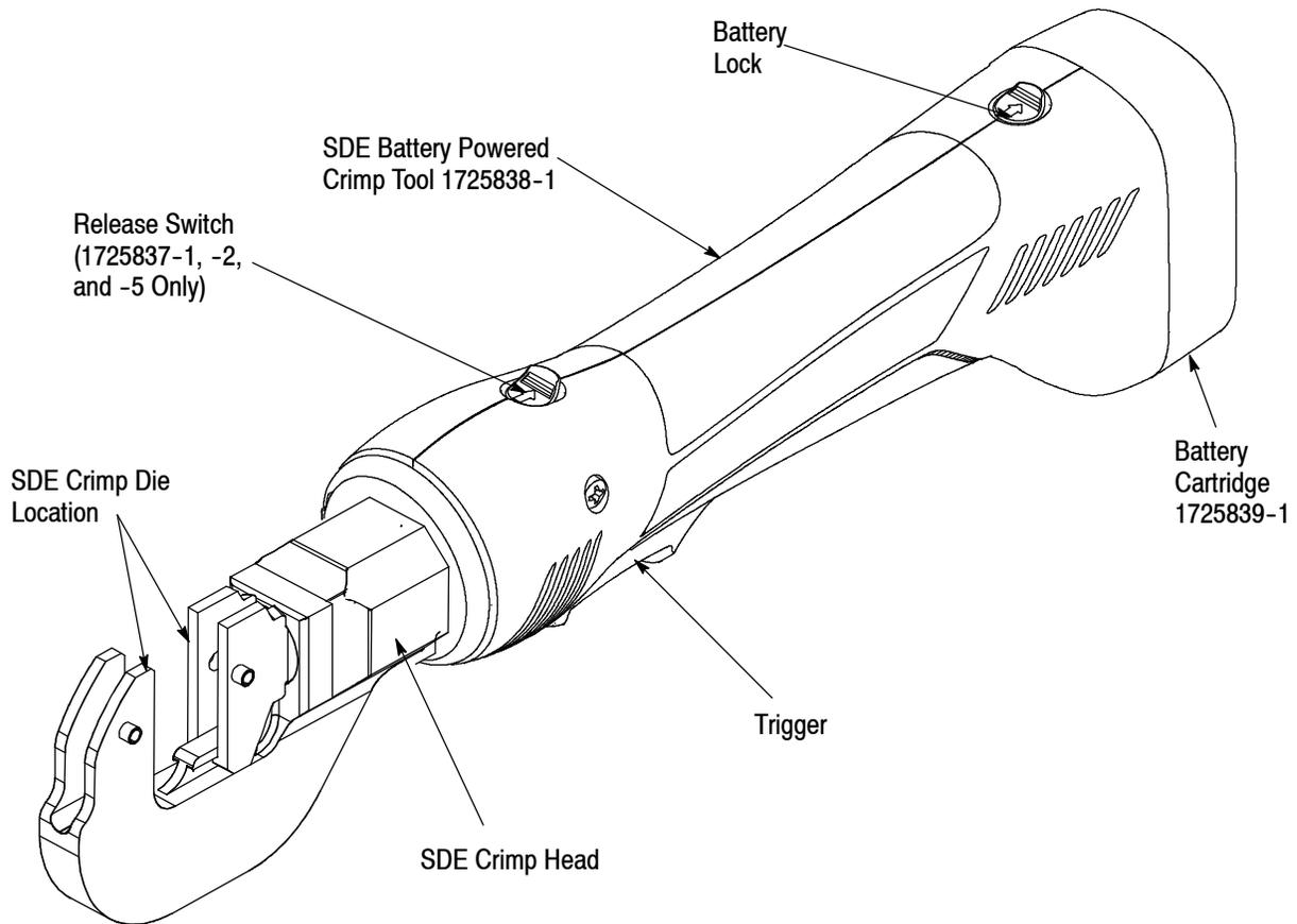
**CRIMPING TOOL (with Battery Installed)**
